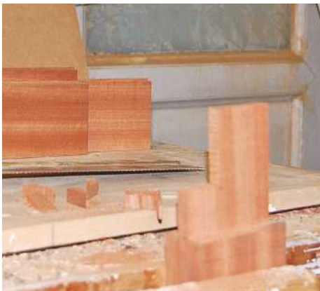
▲ Pic.11 The tenons were haunched to ensure tighter joints
